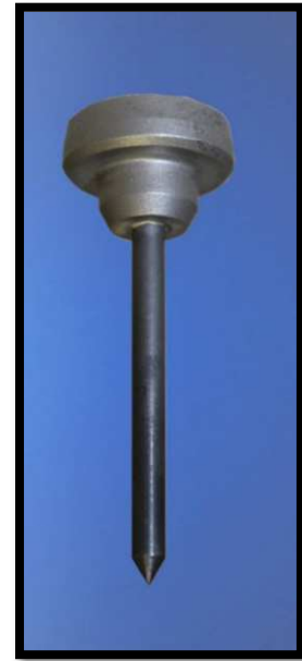
Figure 8 - Close-up of carbide pin
