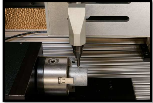
Figure 17 - 3rd axis to mark around part
