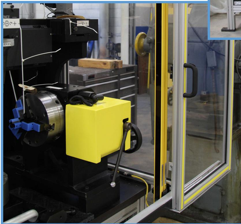
Access doors in the guarding have safety locks. If the doors are opened during the marking cycle, the system will stop.
