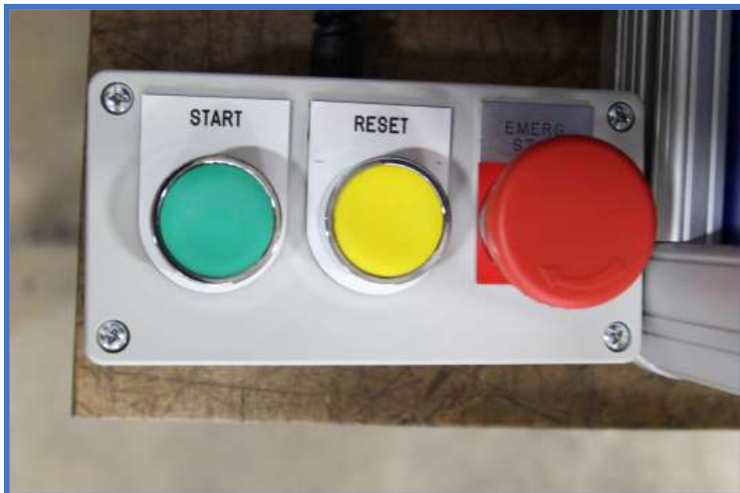
Figure 1 - Automated start feature for CMT Eclipse includes reset, and emergency stop.
